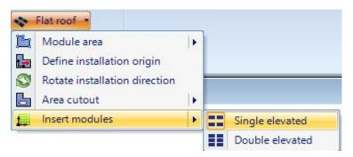
Each time you fill a module area with modules, it will be completely recalculated and previous settings and row spacings are lost.
