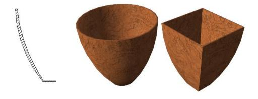
Baluster: On the left the contour and on the right after rotation by 360°, 180° and 270°, respectively.
