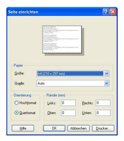
After the dialog has been terminated with 'OK', the printable area is attached to the cursor in the form of a page with the specified values, and can be positioned in the active view, whereby the reference point can be changed with 'Ctrl+w'. The printing process always refers to the view that was active at the start of the process.
