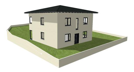
The plot forms a closed 3D solid downwards like the terrain itself. Also with the necessary depth. This prevents a basement, for example, from becoming visible below the surface of the plot.
