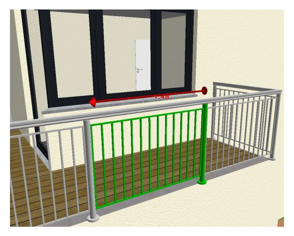
Since changing the length needs a direction in which it should apply, you must first define this direction with a left mouse click on the 3D end of the dimension line. The end of the dimension line also changes its color.
