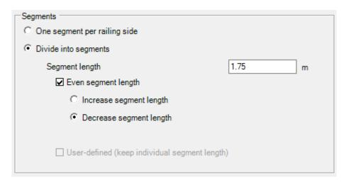
The "Only one segment per railing side" option suppresses the division into segments and creates a railing side with a single segment.
