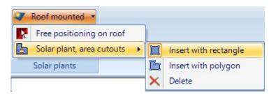
Start the required tool and move the mouse over a module area, which is then labeled and boxed. With a left mouse click in 2D or 3D, select the area and enter the cut-out with your mouse. This action is then only made in 2D views.
