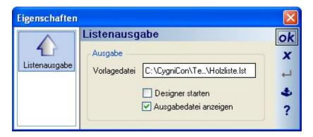
The 'Output list' dialog is terminated with 'OK' and the 'Save report file' dialog is then opened. Here you can enter the desired file name and select the file format from a drop-down list. Normally PDF, RTF, Excel and HTML formats are available.
