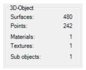
Therefore, depending on the model, always check the number of surfaces, and only create those surfaces that are necessary for the particular application.
