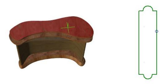
The solid is now created directly with a left mouse-click. The following extrusion solids result for the examples shown.
