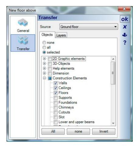
Confirm the settings with 'OK'. You now see the ground floor and the upper floor on top of each other. To show just the upper floor deactivate the ground floor in the project viewer.
