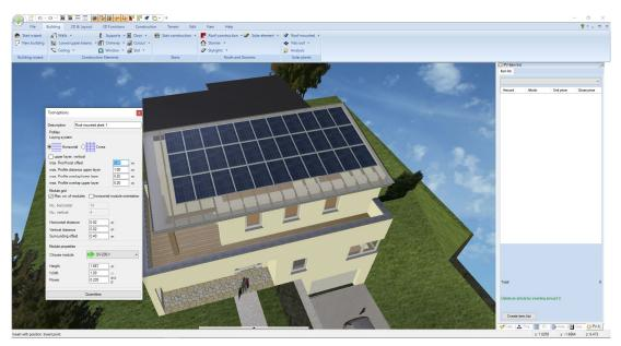
Any changes in the tool option dialog immediately update the preview of the solar system. You can give the plant a unique name for later identification in the reports and bills of quantities and influence the positioning of modules and the mounting system.
