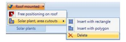
As a module area may contain more than one cut-out, you now need to move the mouse over the desired cut-out which is automatically highlighted. A left mouse click removes it and recalculates the solar plant again.
