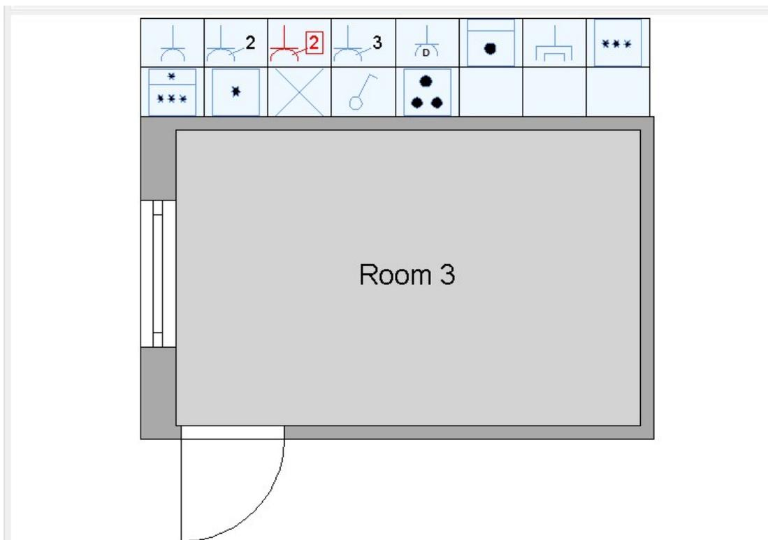
Now, in the preview, left-click on the position on a wall where the socket is to be placed. This will insert the 2D symbol in the preview and remove it from the list.
