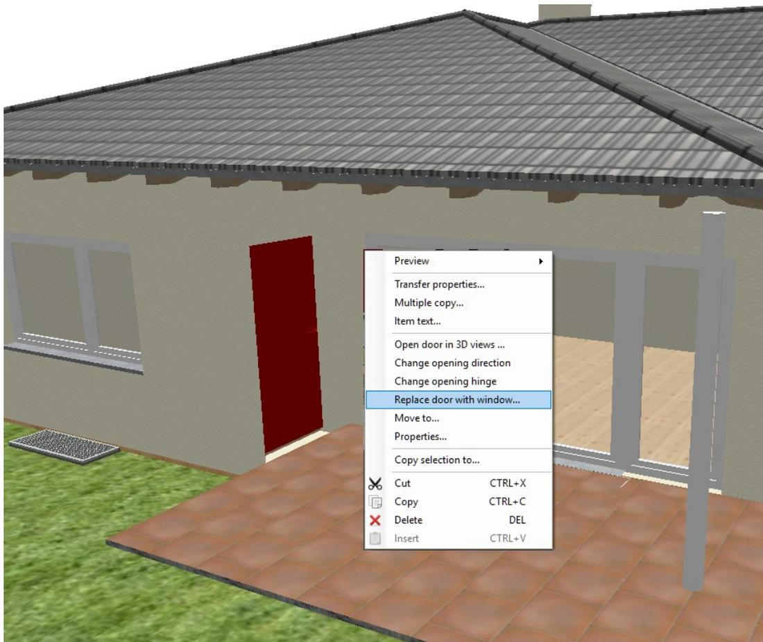
This also works the other way around, i.e. replacing a window with a door.
