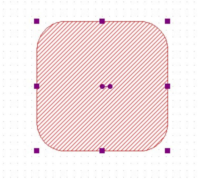
This is exactly the contour that the extrude solids would follow if you try to extrude the rectangle. Since this is not what you want, you would first have to select the rectangle, save it as a 2D symbol in the catalog using the context menu, drag it back into the plan and separate it into its individual objects using the context menu.
