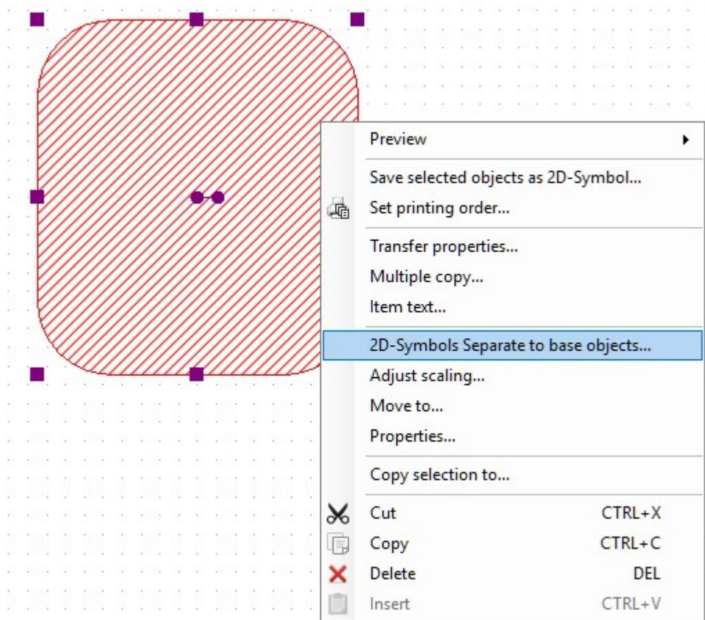
Only now does the former rectangle show the actual contour as a filled 2D polygon and can be extruded in exactly the same way.
